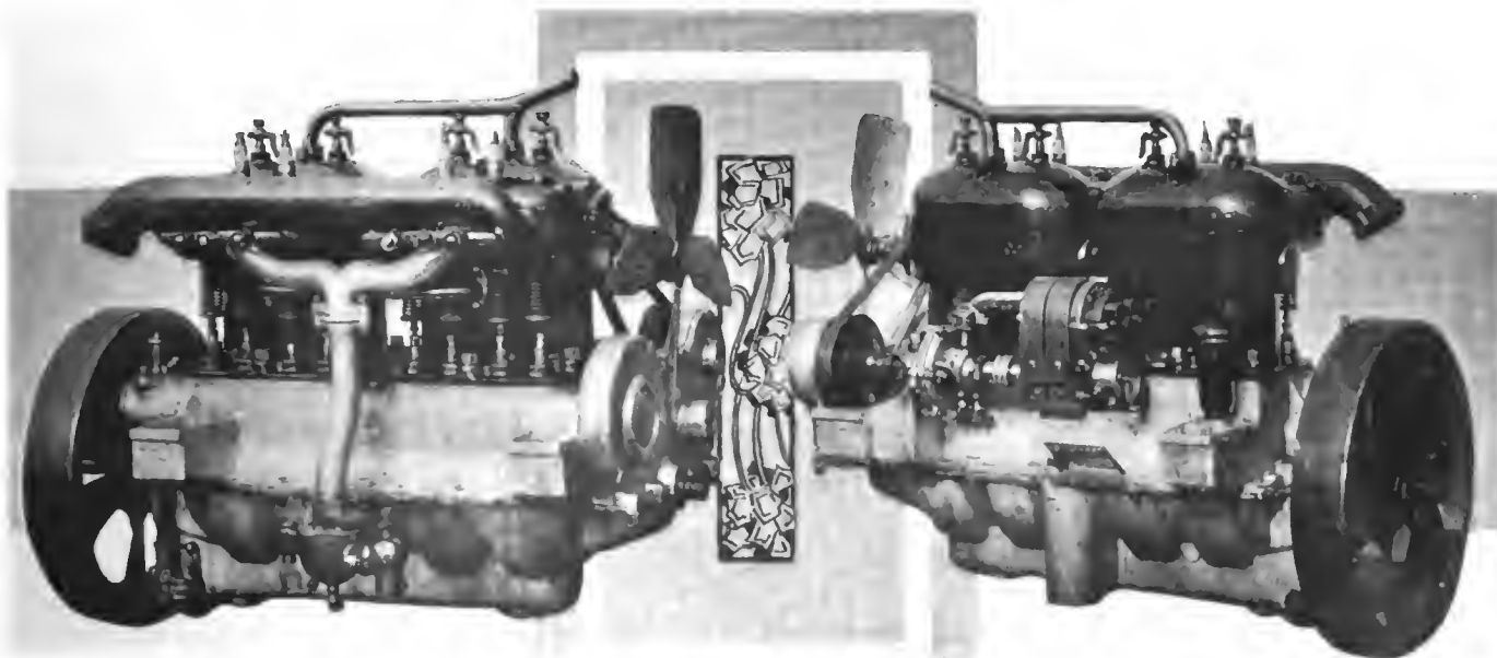
Valve Side of 30-35 Horsepower Engine of Model L Cartercar Accessory Side, Showing Magneto and Pump, Also Fan
